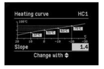
Example: Vitotronic 200 HO1B heating curve
