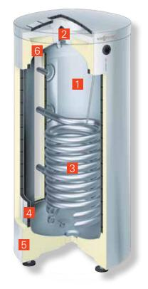
The Vitocell 300-B is a dual mode DHW cylinder with two indirect coils. Made from high alloy stainless steel, the Vitocell 300-B is a reliable and efficient solution for the integration of two energy sources. Available in two sizes, either 300 litres or 500 litres.
